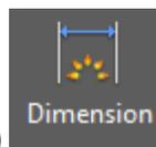
11. Dimension (**DIM Space**) to Create linear or aligned dimension.
